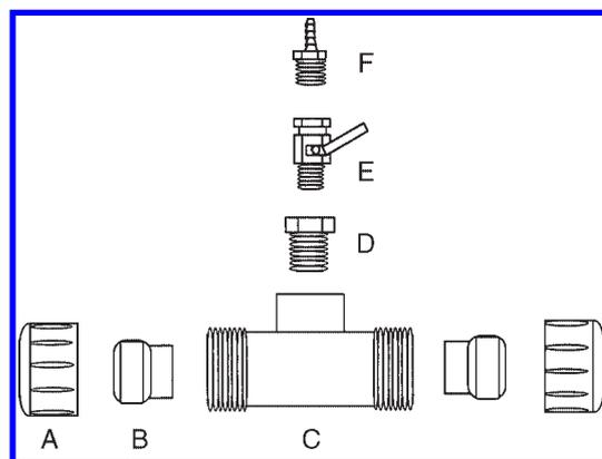
Figure 1. Schematic of PVC cell. Parts A, B, and C comprise the body of the cell. Two NaCl windows are securely positioned in the compression fittings (B) using a short segment of PVC tubing. A  $\frac{1}{2}$ - to  $\frac{1}{4}$ -in. PVC bushing (D) serves as the adapter to connect a ball valve (E) to the tee. A suitable adapter (F) is connected to the valve.
