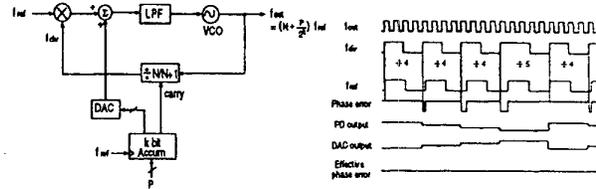
Figure 1. Fractional-N frequency synthesizer ( $N_{eff}=4+1/4$ ).
