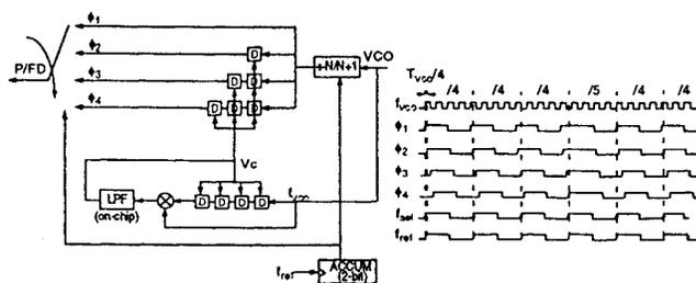
Figure 3. Phase compensation with on-chip tuning (modulo=4).
