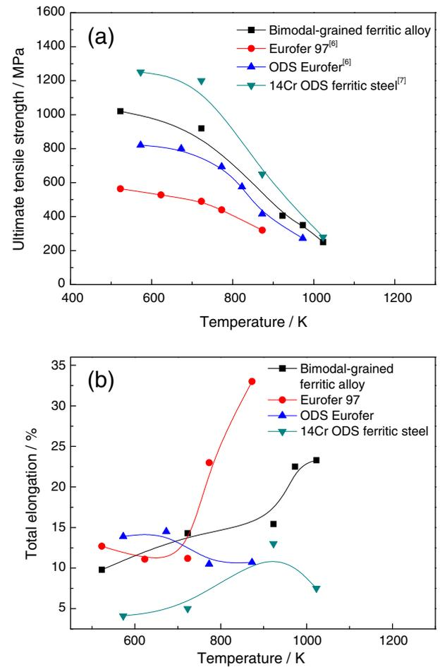
**Fig. 2.** Mechanical properties of the bimodal-grained ferritic alloy: (a) ultimate tensile strength vs. test temperatures and (b) total elongation vs. test temperatures.
