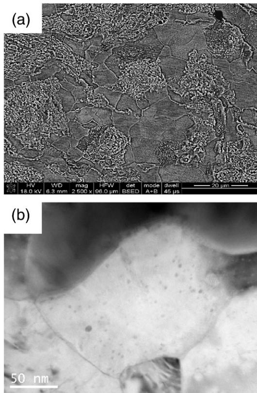
**Fig. 1.** Microstructure of the as-annealed ferritic alloy with a bimodal grain structure: (a) SEM image of both nanometer-sized fine grain region and micron-sized coarse grain region and (b) bright field TEM image of the nanometer-sized fine grain region.
