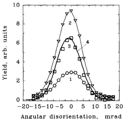
Fig. 10. Orientation dependencies of PXR from the crystal, curve 1, and X-rays from a compound target, curve 2, measured at the extracted beam of the Tokyo synchrotron. Curve 3 shows the orientation dependence of DRTR. Curve 4 is the calculated orientation dependence of DRTR.
