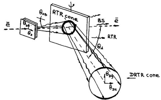
Fig. 3. Scheme of RTR photons reflection by a crystal.
