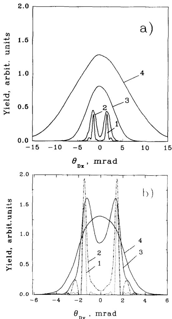
Fig. 5. (a) Diffracted RTR intensity as a function of the emission angle  $\theta_{Dx}$  at fixed emission angle  $\theta_{Dy} = 0$ ; (b) DRTR intensity as a function of  $\theta_{Dy}$  at  $\theta_{Dx} = 0$ . Curves 1, 2, 3 and 4 correspond to the crystal mosaicity  $\sigma_m = 0.1, 0.3, 1.0$  and  $3.0$  mrad, respectively.
