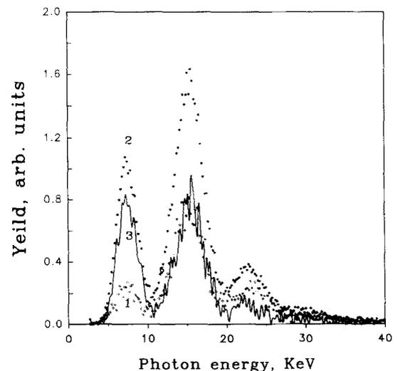
Fig. 9. Experimental spectra of PXR from a pyrolytic graphite crystal, curve 1, and X-rays from a compound target, curve 2, obtained by using the extracted 900 MeV electron beam of the Tokyo synchrotron.
