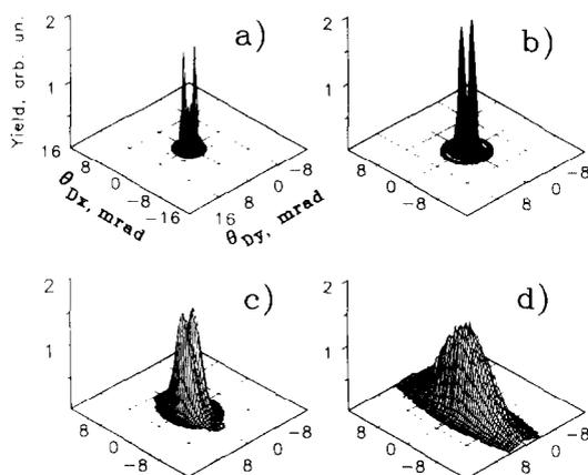
Fig. 4. Calculated angular distribution of RTR photons reflected by pyrolytic graphite crystals with mosaicity (a)  $\sigma_m = 0.1$ ; (b)  $\sigma_m = 0.3$ ; (c)  $\sigma_m = 1.0$ ; and (d)  $\sigma_m = 3.0$  mrad.
