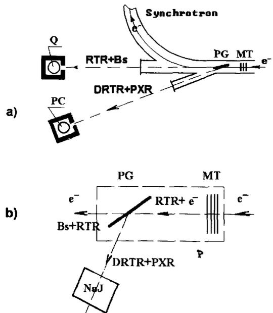
Fig. 7. Experimental arrangements at the Tomsk (a) and the Tokyo (b) synchrotrons. MT = multifoil target, PG = crystal, Q = quantometer, PC = proportional counter, P = iron plate for the mounting of MT and PG in the goniometer, NaI = scintillation spectrometer, Bs = bremsstrahlung.
