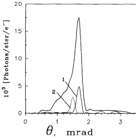
Fig. 2. Calculated angular distribution of RTR photons with energies of 5–30 keV (the upper curves). Curves 1 and 2 show the angular distributions of the photons forming RTR spectrum into energy ranges 1 and 2 (see Fig. 1).
