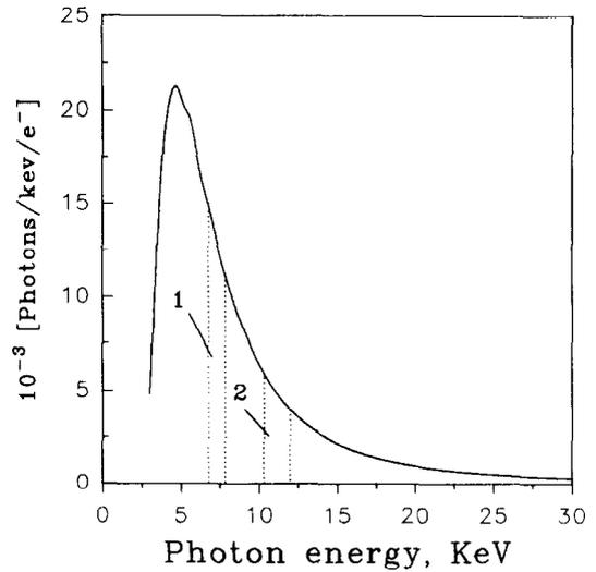
Fig. 1. Calculated spectrum of RTR generated by 900 MeV electrons in the 10 Mylar foil target ( $l_1 = 12 \mu\text{m}$ ;  $l_2 = 52 \mu\text{m}$ ).
