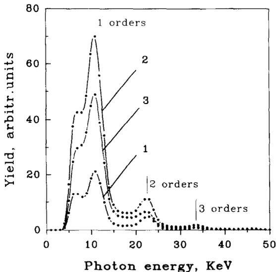
Fig. 8. Measured spectra of PXR from a pyrolytic graphite crystal, curve 1, and X-rays from a compound target, curve 2, generated by 900 MeV electrons of the internal beam of the Tomsk synchrotron. Curve 3 is the DRTR spectrum.
