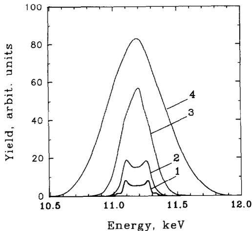
Fig. 6. DRTR spectrum versus the crystal mosaicity. Curves 1–4 correspond to  $\sigma_m = 0.1, 0.3, 1.0$  and  $3.0$  mrad, respectively.
